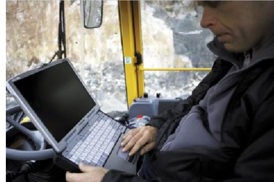
MATRIS stores operational data and shows how the machine is working. This provides valuable information for fault-tracing and service.
